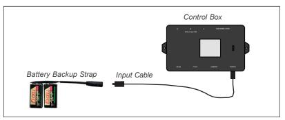
**Note:** Detach the Battery Backup Strap after the emergency is over, as the system will continue to draw power from the batteries even if not in use.
