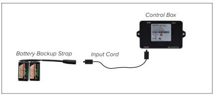
**Note:** Detach the Battery Backup Strap after the emergency is over, as the system will continue to draw power from the batteries even if not in use.
