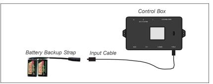
**Note:** Detach the Battery Backup Strap after the emergency is over, as the system will continue to draw power from the batteries even if not in use.
